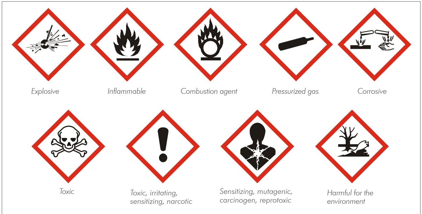
Figure 2 : Symbols of chemical risks New pictograms of European Regulations – GHS (Globally Harmonized System).
