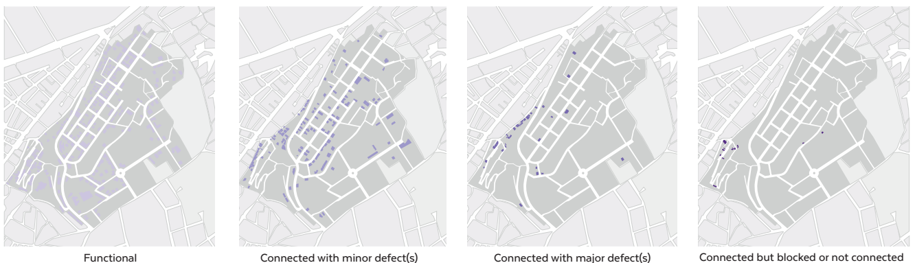
Figure 46 Condition of buildings' connection to wastewater network
