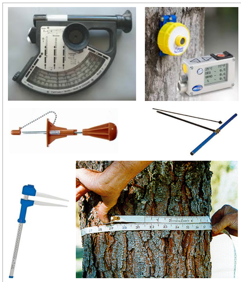
Figure 15. Equipment for dendrometric data collection (A- Blume-Leiss hypsometer, B- Vertex hypsometer, C- Bark thickness gauge, D- Increment borer, E- Caliper, F- PI tape)
