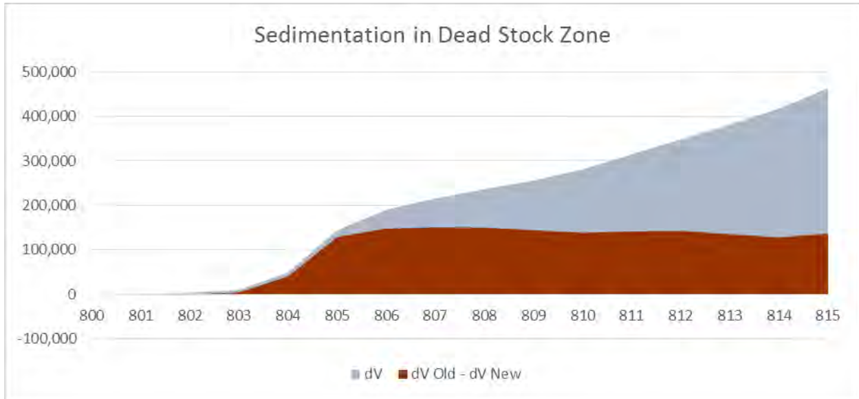
Figure 11 Graph showing the sedimentation volume compared to the original storage capacity in the Dead Stock Zone (below 815 mASL)
