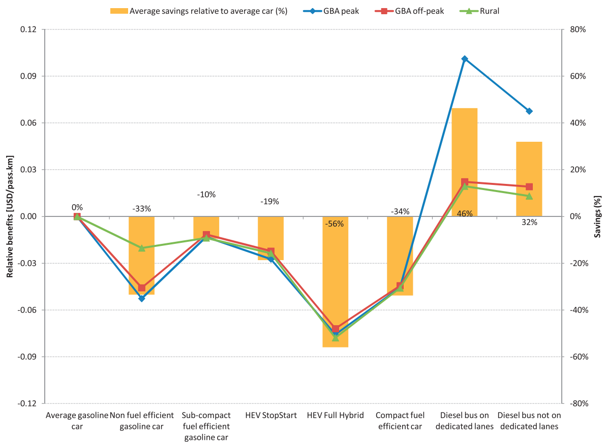
Fig. 44 - Government benefits of transport technologies relative to average car under GBA driving conditions.
