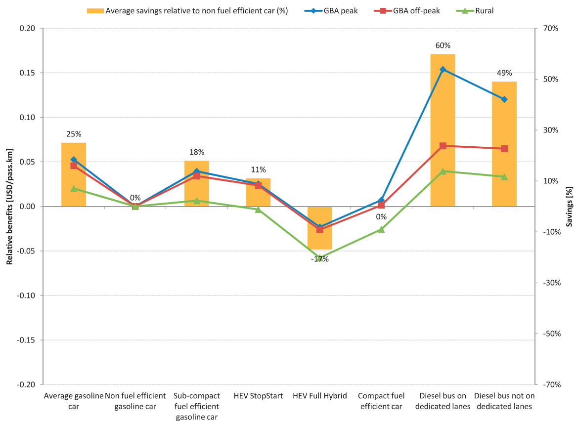
Fig. 45 - Government benefits of transport technologies relative to non fuel efficient car under GBA driving conditions.
